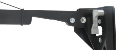
The compact 050-7130 10mm Single Rotor Latch with Squeeze Release is designed for operator door applications for off-highway vehicles that require a remote interior release. Similar to the 050-7120, this 10mm Single Rotor Latch with Direct Squeeze Release allows inside squeeze release integration into the customers door tubing.
